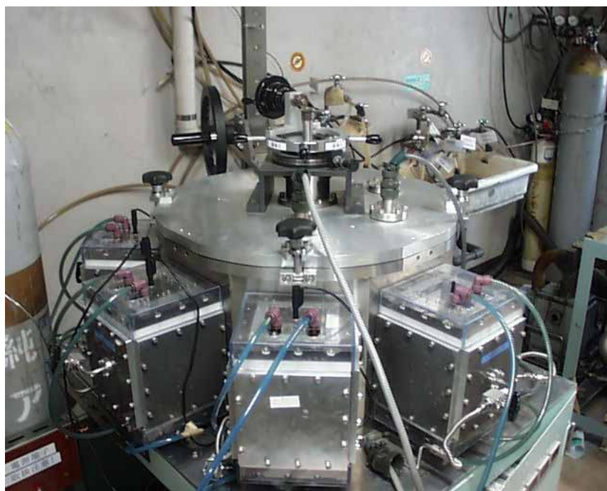
Fig. 3.3 Facing targets sputtering apparatus for multilayered thin films.
