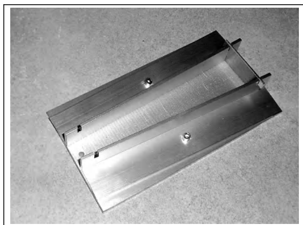
Figure 1c – Photo of support used for cyclic mechanical movement of sealant
