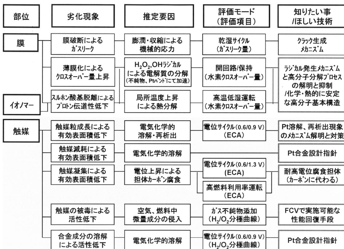
Fig. 1.3.3 Possible MEA degradation map for FCV<sup>13)</sup>.
