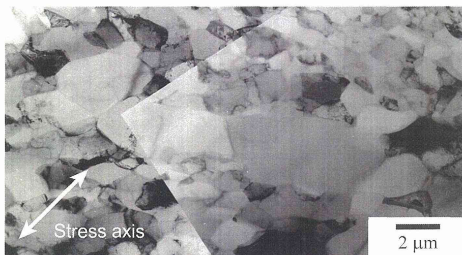
Figure 4-5. Occurrence of local grain coarsening in a specimen fatigued at 198 K.
