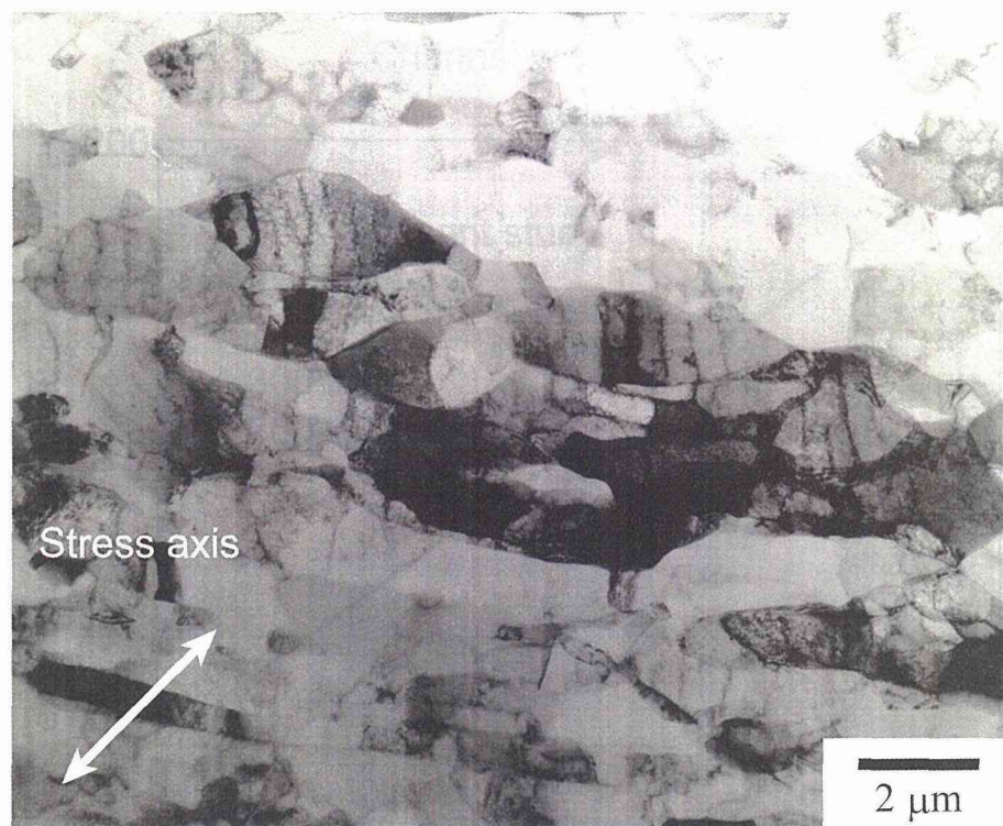
Figure 4-8. TEM photograph of UFG Al fatigued at 83 K. The fraction of grains that contain dislocation wall structure is about 50 %.
