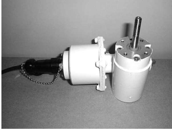
Figure 4.7: A stepping motor (Oriental Motor PX533MH-A) for adjustment of mirror direction.
