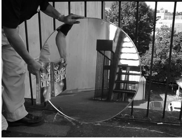
Figure 4.6: A spherical mirror of the CANGAROO-II telescope.
