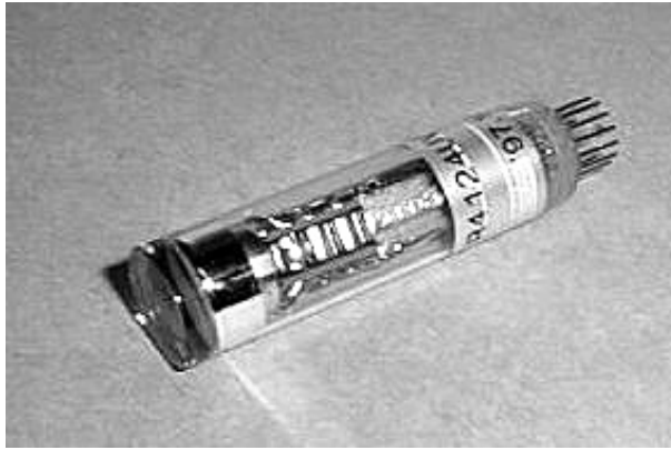
Figure 4.10: PMT Hamamatsu R4124UV, of which diameter is 13mm and length is 50mm.
