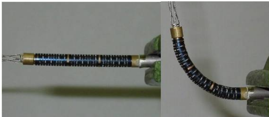
Fig. 1.26: Flexible distal mechanism made of a super-elastic tube (Peirs et. al.) [91]
