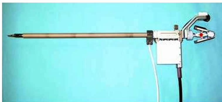
Fig. 1.3: Hand-held type robotic forceps [15]
