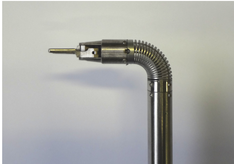
Fig. 2.5: The flexible joint bent by 90°
