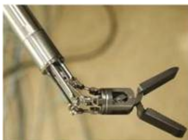
Fig. 1.20: Forceps manipulator with parallel mechanism (Hong et. al.) [59]
