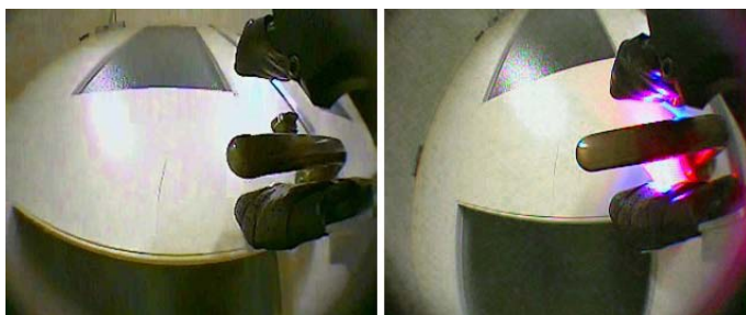
Fig. 7.17: Gripper camera view without LED(left), with LED(right)
