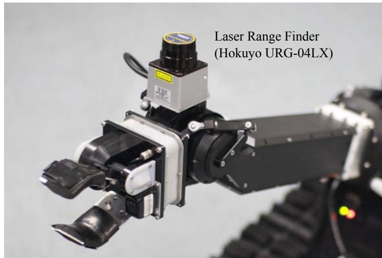
Fig. 7.7: Laser Range Finder on the wrist
