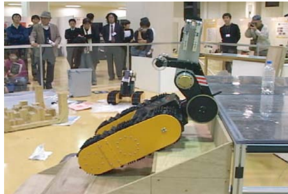
Fig. 2.8: HELIOS VIII- stairs climbing test
