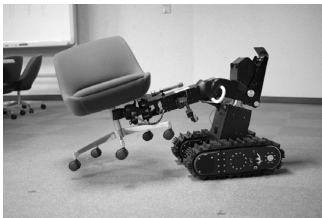
Fig. 8.10: Lifting a 7 kg chair
