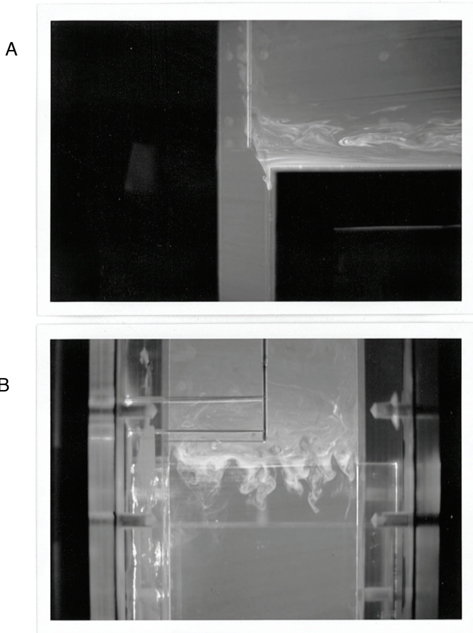
Fig. 3.2-8 Photos of Penetration Flow
