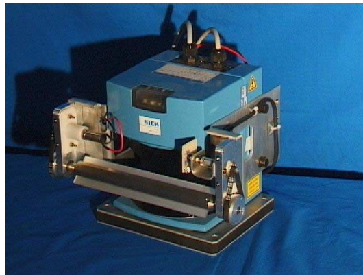
Fig. 2.26: Laser Range Finder "Sick LMS200" and the pitching scan mechanism
