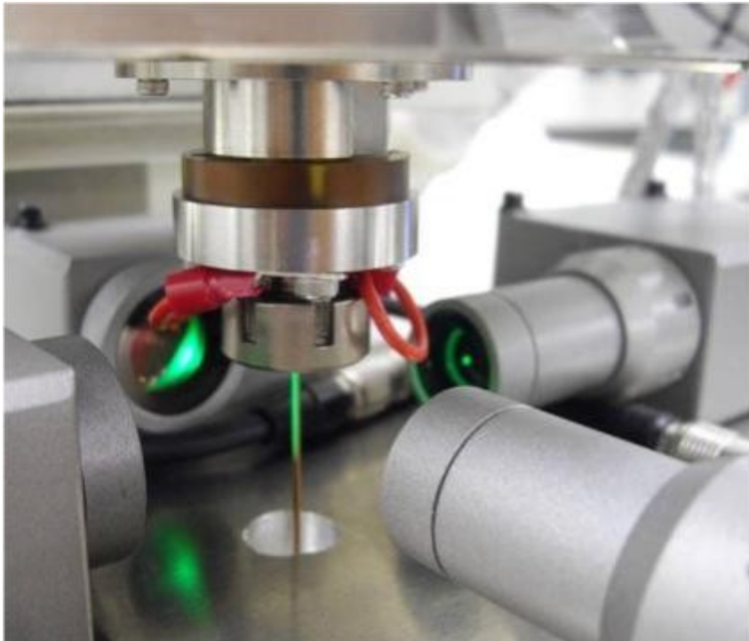
Fig. 3.7 Measurement of electrode rotational accuracy
