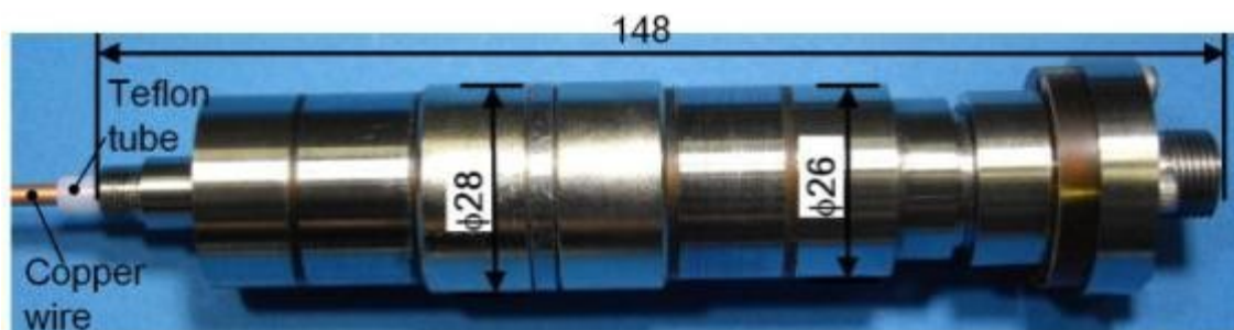
Fig. 3.6 Spindle shaft and electrode attachment (new type)
