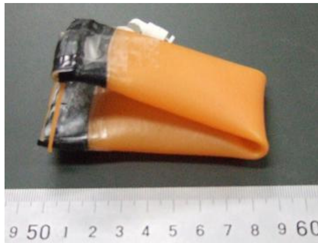
Fig.2-9 A S/A bag with elastic body for linear actuator
