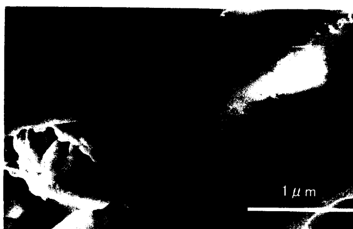
Fig.3-3 SEM photographs of H + -mordenite-HSBR composite membranes.
