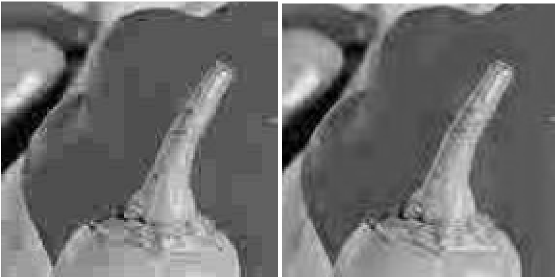
Figure 1.2: Difference of decoded images with the DCT (left) and the lapped transform (right): the decoded image with the lapped transform contains ringing artifacts around edges caused by long basis functions
