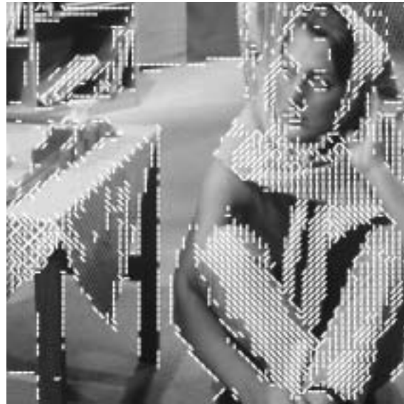
Figure 5.7: Classification map of “Barbara” in the Type-E coder: Each white line indicates the angle of the directional block.
