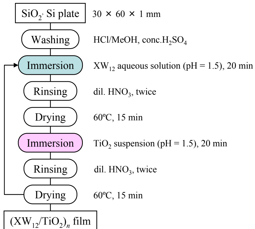
Figure 4-5. Experimental procedure of (XW 12 /TiO 2 ) n thin film preparation using LBL method.
