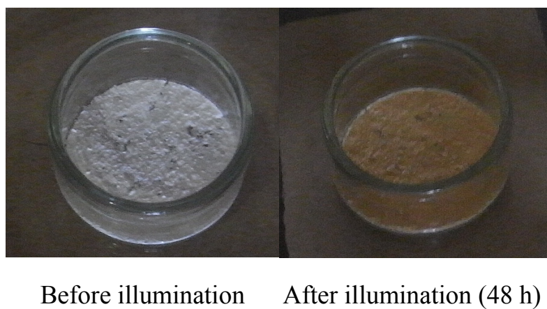
Figure 6-9. Sample color change after illumination. Sample: hybrid-1, 1 mW/cm 2 light intensity (365 nm).
