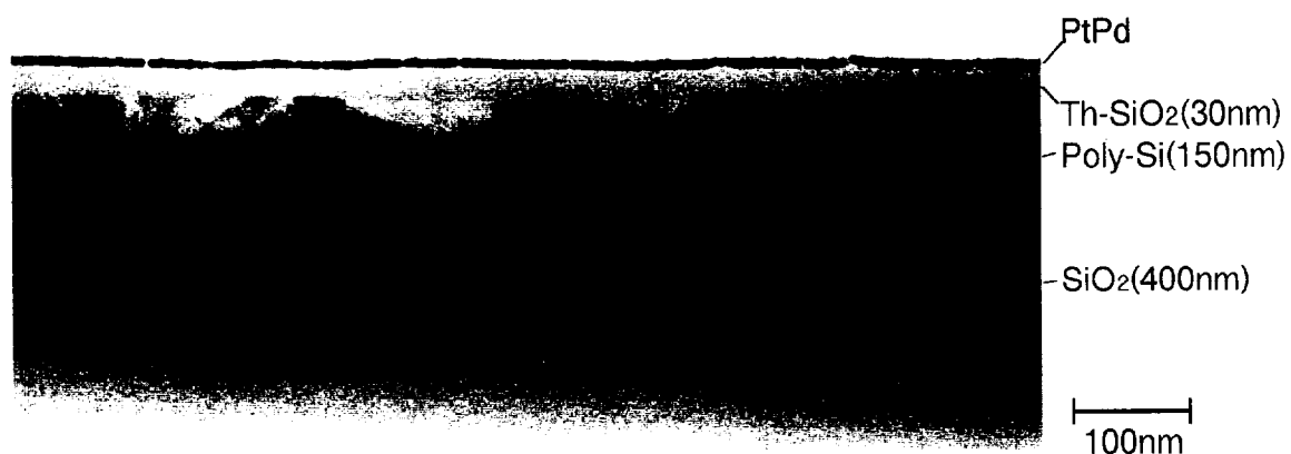
Fig. 2.80 TEM micrograph of cross section of SiO 2 -poly-Si interface.
