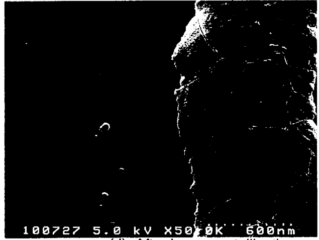
(d) After laser crystallization at 400 mJ/cm², 350°C
