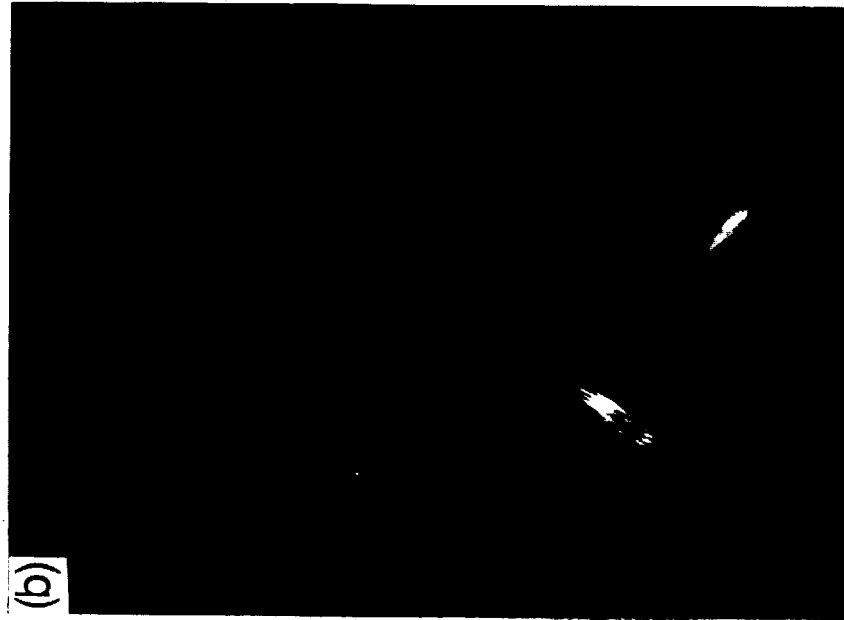
Fig.2-37 Transmission electron micrographs after aging at 773K for 250ks in a Cu-4mol%Ni-4mol%Si alloy. (a)diffraction pattern, (b)dark field image of plate-like phases,(c)dark field image of spherical phases.
