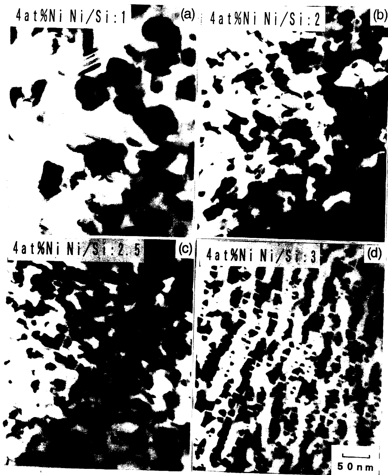
Fig.2-32 Transmission electron micrographs after aging at 773K 72ks. (a)value of Ni/Si is 1, (b)value of Ni/Si is 2, (c)value of Ni/Si is 2.5 and (d)value of Ni/Si is 3.
