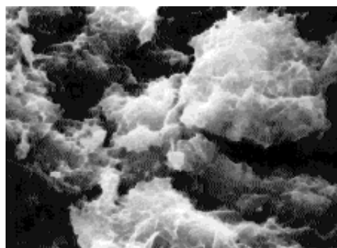
(4) WSL autoclave curing at 180°C
