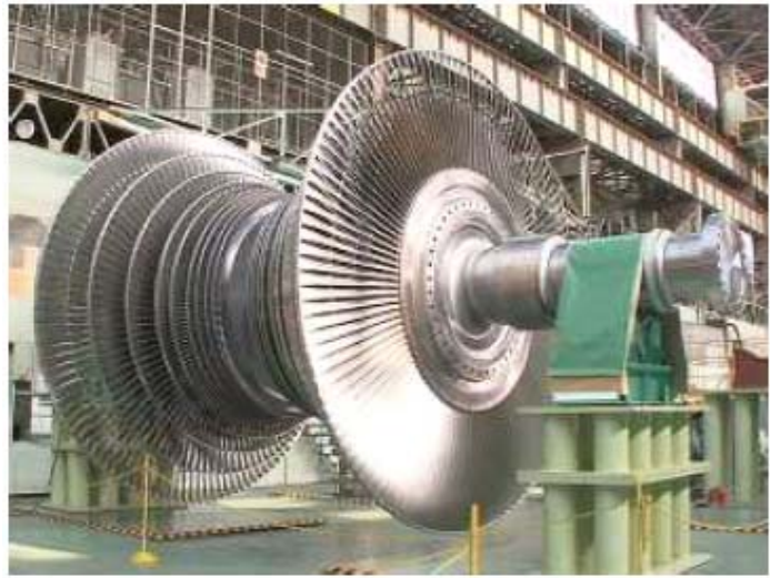
(b) Low pressure turbine with 54 inch length last stage blade
