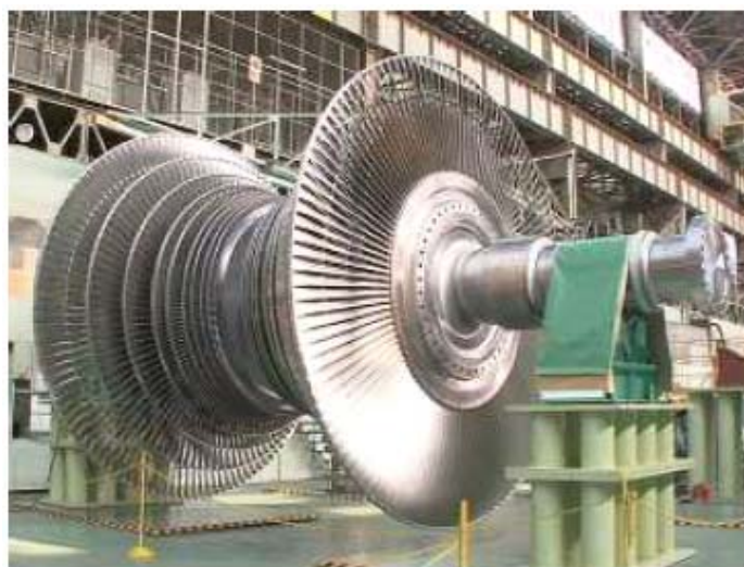
(b) Low pressure turbine with 54 inch length last stage blade
