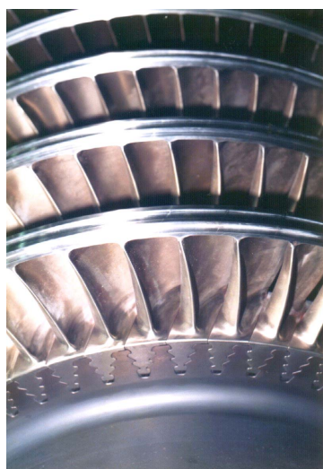
(a) Three dimensional flows designed Integral shroud blade (ISB)
