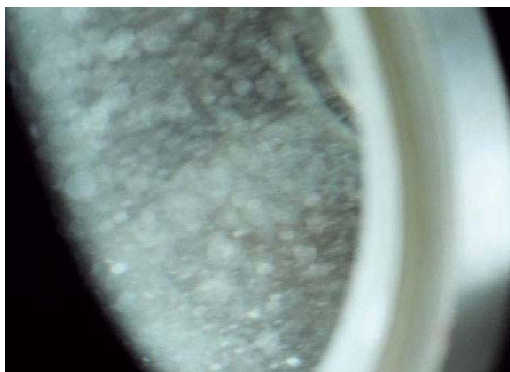
(a) Visualized data at room temperature with saturated air, NPSH_{av} = 7.93 m, rated flow
