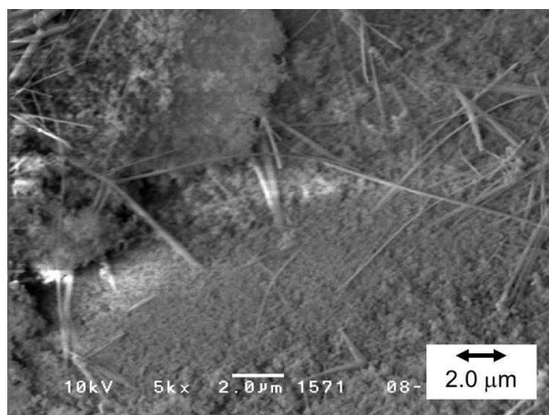
Figure 5.3-18 SEM micrograph of \text{LiCl/Mg(OH)}_2 ( \alpha = 0.10 ) after 105 runs. The graph is magnified a 5000 times.
