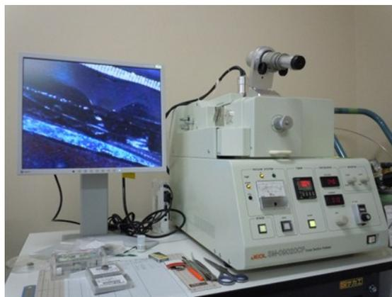
Figure 3-8. Cross-section polisher.
