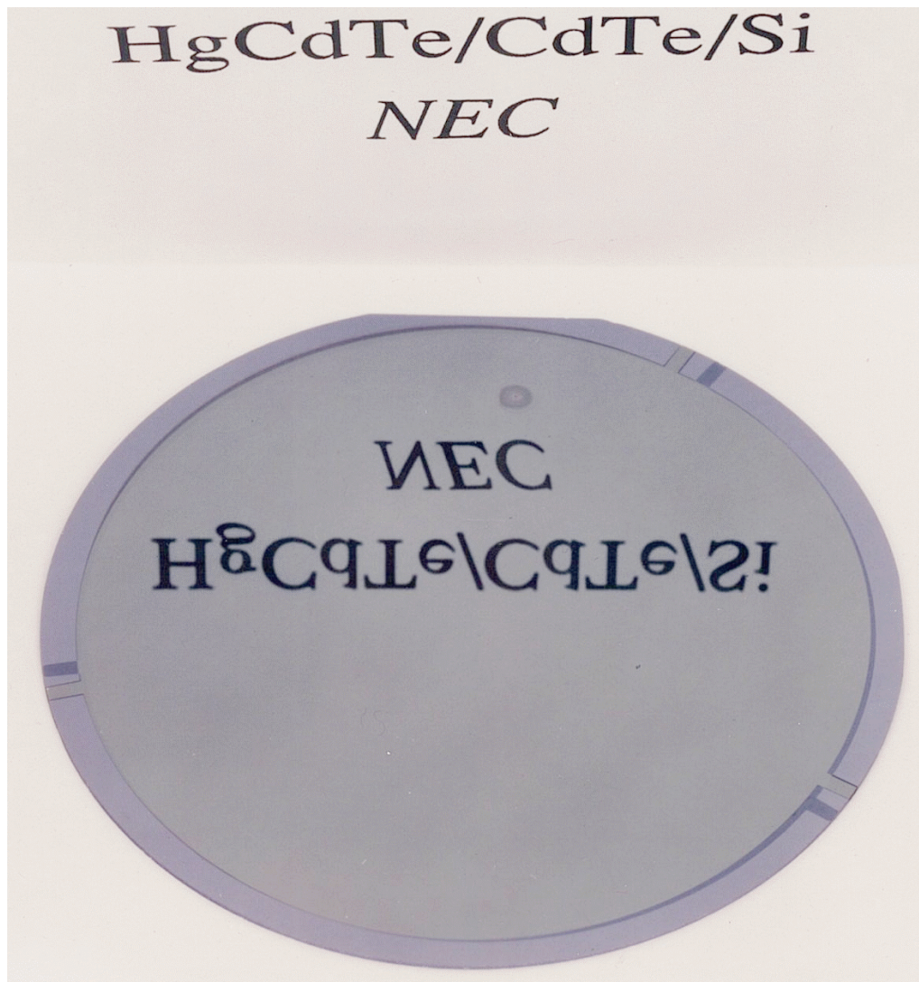
Fig. 2-21 External view of MBE grown HgCdTe surface on 3 inch Si wafer. Mirror-like surface morphology was obtained.
