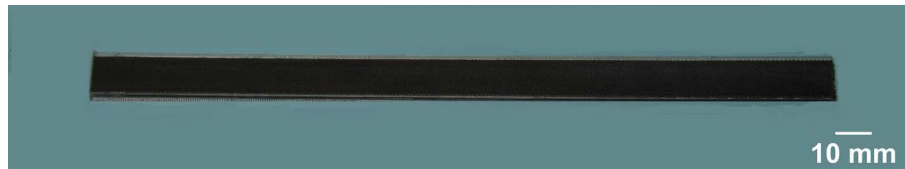
Figure 5. Sample with 6 layers of CFRTTP printed by the Mark One ® . The sample still has to be ground and the tabs still have to be attached.
