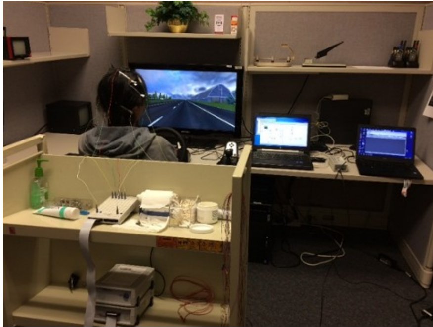
FIGURE 7.2: Preliminary study on EEG/EOG-based human fatigue measurement while engaging self-driving simulator. The study was conducted at Fatigue Countermeasures Group, Human Systems Integration Division, NASA Ames Research Center
