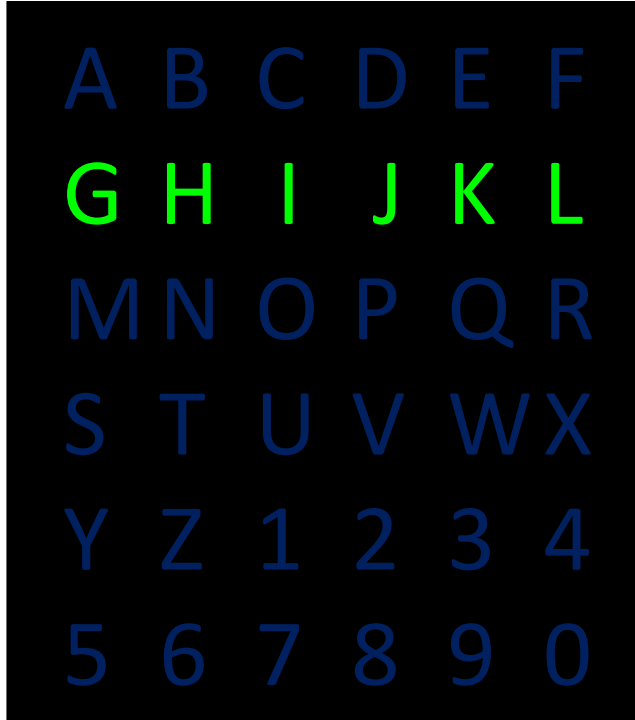
FIGURE 2.4: The P300 speller with row/column green/blue flickering matrix
