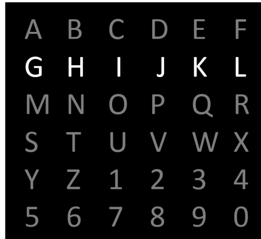
FIGURE 1.3: Illustration of the conventional P300-Speller capture screen.
