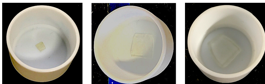
Figure 3-15. RCP 70 (left) in dry state, (middle) swollen with DMSO, (c) after being heated at 140 °C for 1 month.
