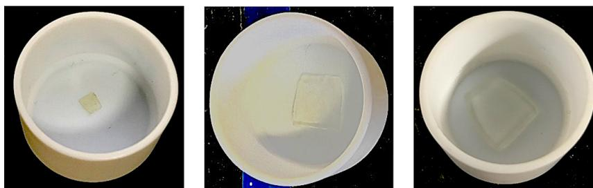
**Figure 3-15.** **RCP<sub>70</sub>** (left) in dry state, (middle) swollen with DMSO, (c) after being heated at 140 °C for 1 month.
