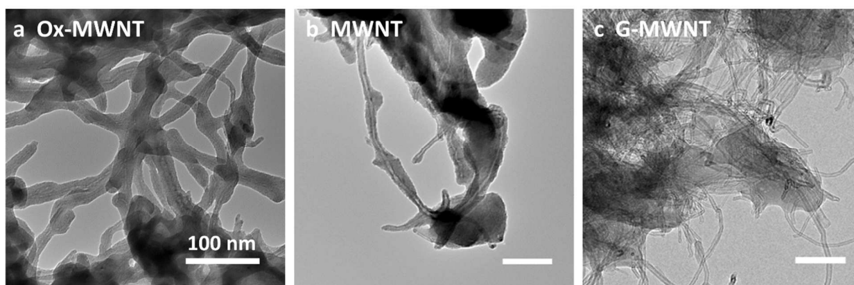
Figure 3.6 - TEM characterisations of DC product morphology at 1 mAh (a) Ox-MWNT (b) MWNT and (c) G-MWNT following DC to 1 mAh at current rate of 50 \text{ mA g}^{-1} . The scale bars indicate 100 nm.
