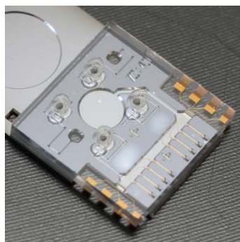
Fig. 5.30 Anodic bonded silicon fluidic chip with glass having electrodes
