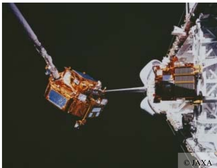
Fig. 2-6. SFU spacecraft captured by the robot arm of the space shuttle.
