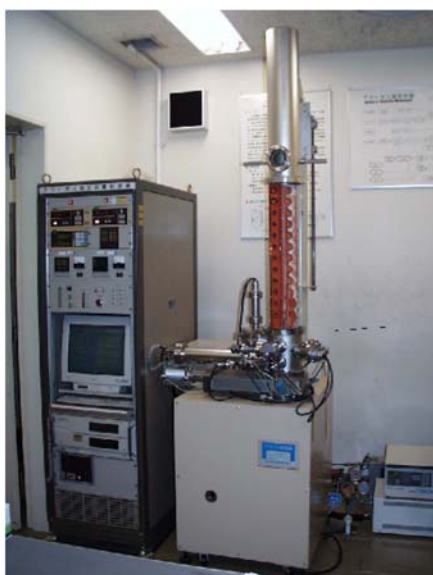
Fig. 1-7. Outgas Measuring System.
