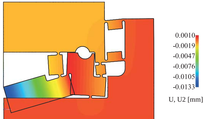
Fig. 3.9: Contour plot of the calculated displacement U_2 of the displacement magnifier. Applied rotor deformation is 1\text{ }\mu\text{m} between the top face. Rotor deformation is magnified approximately 12 times at the left surface. Displayed displacement is magnified 100 times.
