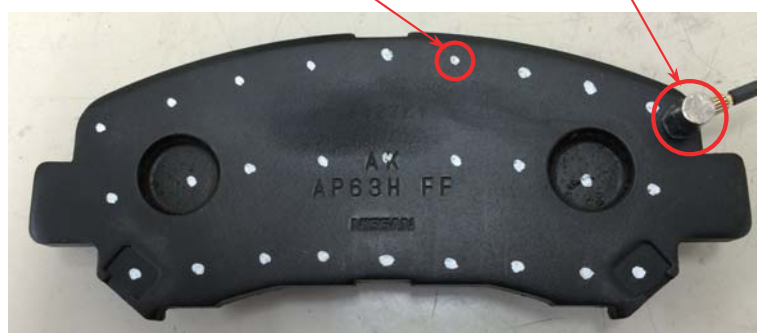
Fig. 2.11: Impact points and measurement point of the brake pad. Mode shapes are measured with hammering at multiple points (white dots in this picture.)
