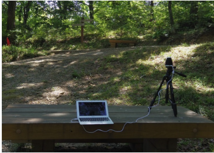
Figure 5.4: Recording system with a microphone array
