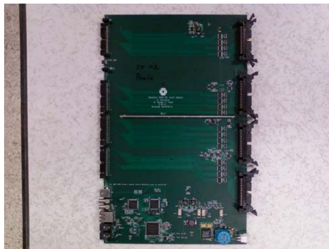
Figure 3.26: Level Shifter Board. The Level Shifter Board receives the signals from ASDQ cards from the right side of the picture. After processing, the Level Shifter Board sends LVDS signals from the left side.
