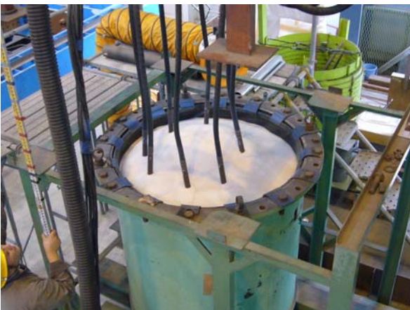
Photo 2.7 Vibration to the sand deposit
