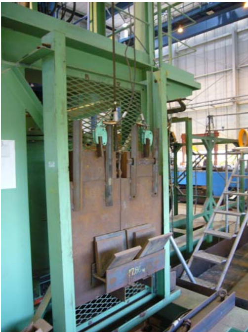
Photo 2.19 Adjustment of applied load acting on pile head
