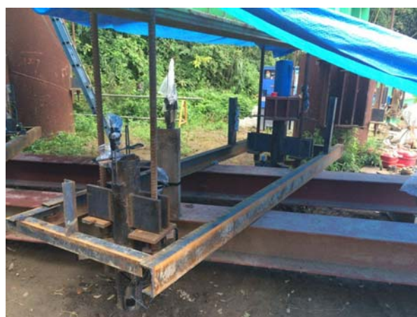
Photo 5.6 Monotonic tensile loading (B-MT)
