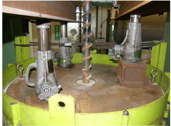
Photo 2.23 Loading overburden pressure
