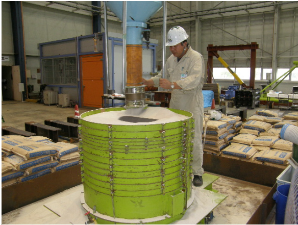
Photo 2.22 Pluviating sand into the tank
