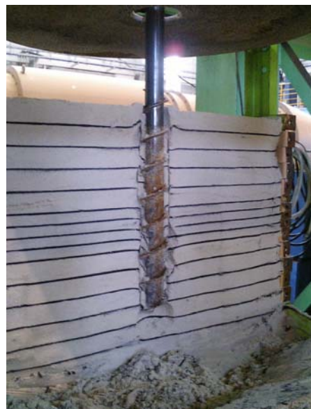
Photo 2.27 Loading on pile head
