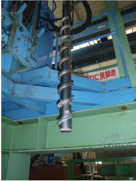
Photo 4.1 Continuous helix pile
