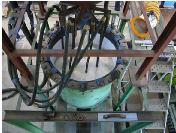
Photo 2.6 Sand pluviated into the tank
