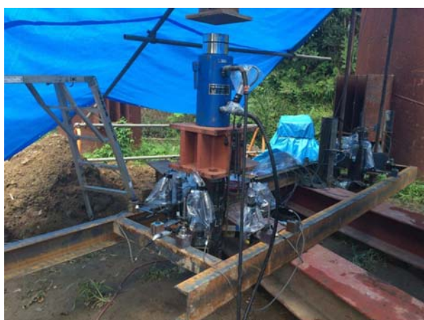
Photo 5.5 Monotonic compressive loading (B-MC)
