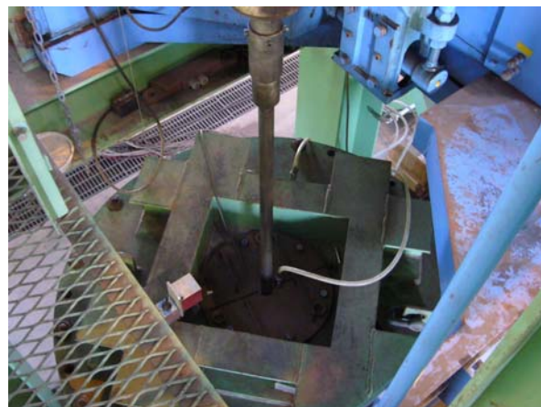
Photo 2.15 Cone penetration test
