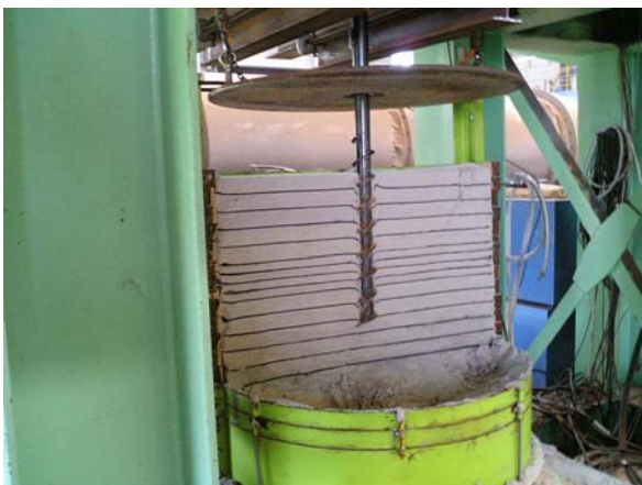
Photo 2.26 Section of sand tank
