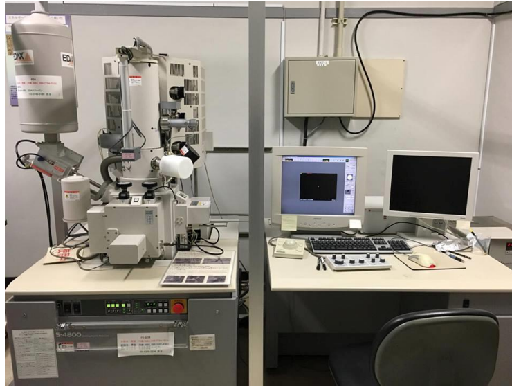
Fig. 3.6 Appearance of the SEM-EDX instrument used for microstructure analysis.
