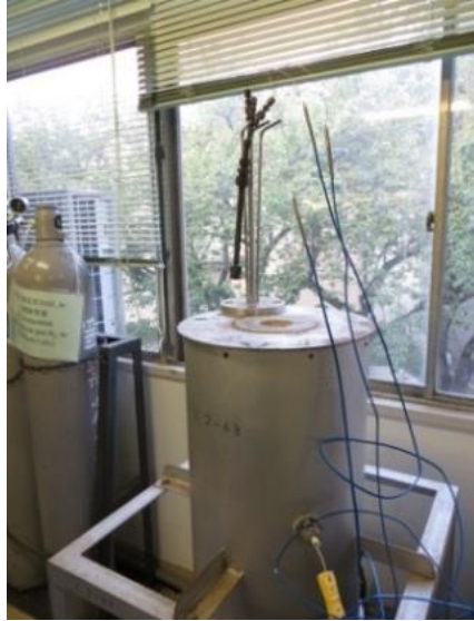
Fig. 2.8 Outside view of high-temperature furnace which is used for diffusion.
