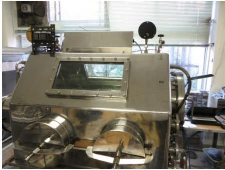
Fig. 2.6 Outside view of glove box which is used to melt the solid LBE and Pb-17Li, then manufacturing the liquid lead alloy into a capillary.
