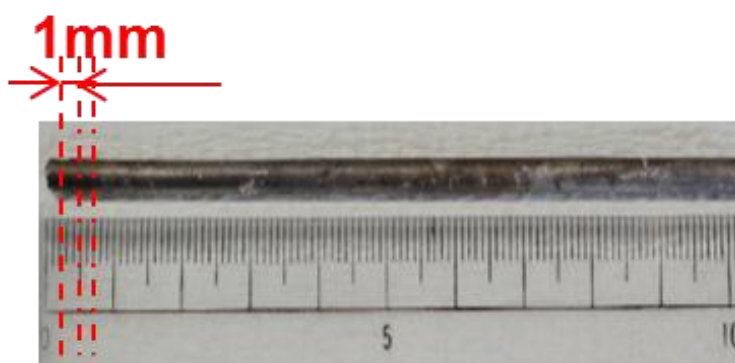
Fig. 2.12 The solid specimen after the diffusion experiment and it is cut into 1mm per piece.
