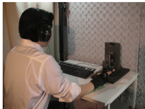
Fig. 1 Experimental environment. A sinusoidal wave sound was presented to the participants through earphones. The haptic device was attached to the right index finger of the participants. Under the involuntary movement condition, the haptic device moved their right index finger.
