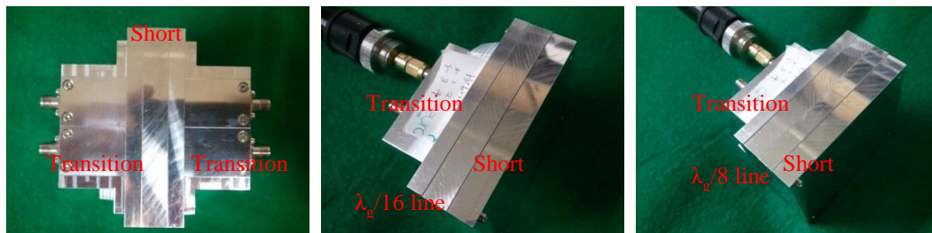
Fig. 3.13 RLL calibration (a) Reflect (b) Reflect with \lambda_g/16 line (c) Reflect with \lambda_g/8 line.
