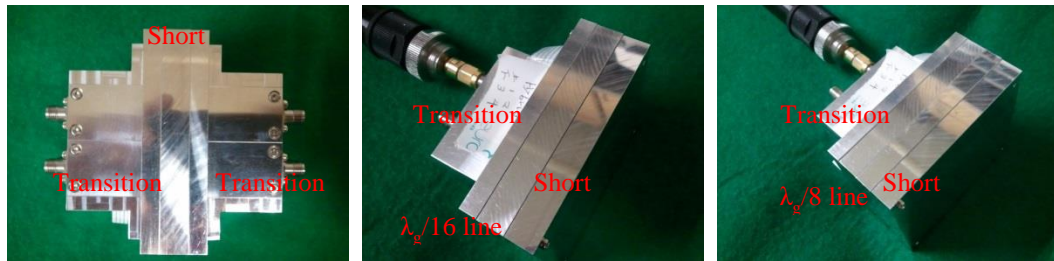
Fig. 3.13 RLL calibration (a) Reflect (b) Reflect with \lambda_g/16 line (c) Reflect with \lambda_g/8 line.
