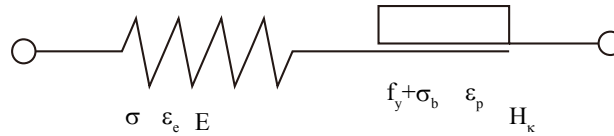
Fig. 3.16. A series model representing the bilinear behavior of the BRC hinge
