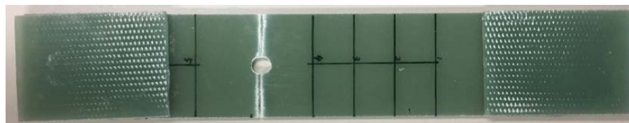
Figure 2.3 Glass-fiber-reinforced plastic specimens after tensile testing
