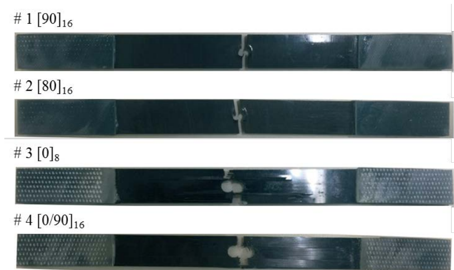
Figure 2.2 Carbon-fiber-reinforced plastic specimens after tensile testing
