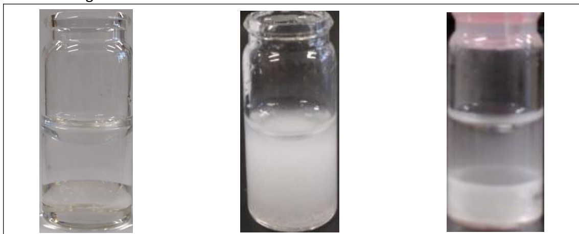
Figure 4-8 Mixing results of benzene-guaiacol-water (Before shocking: left, After shocking: middle, Standing for 1 hour: right )
