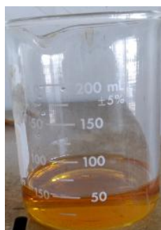
Figure 4-6 The harmonious state of CD cracked oil/biodiesel=1:50
