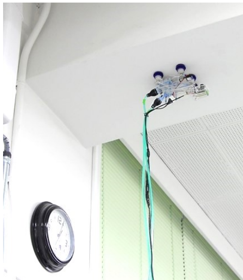
Figure 2.17 Attachment condition and robotic movement with upside down condition
