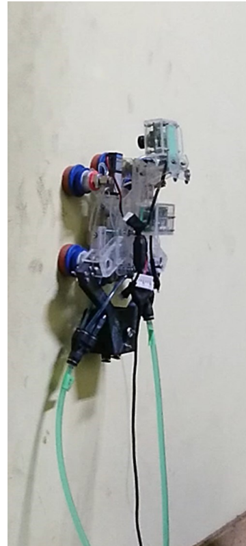
Figure 4.46 Movement performance on a corroded metal surface and concrete wall surface, (a) Corroded metal surface, (b) Mortar wall surface
