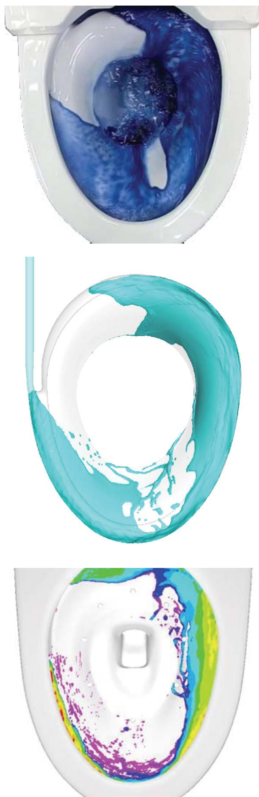
図 6.17 The comparison of the result of present method (middle) and our existing method using Cartesian grid (lower) with the experimental result (upper).
