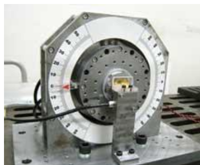
Fig. 1.2: Pneumatic rotary actuator system using an electromagnetic force by Shinno and Yoshioka (33)
