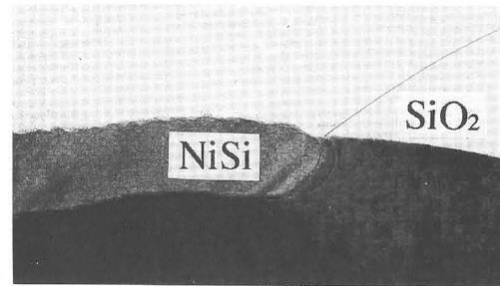
Fig. 2-2-2. TEM photograph of NiSi film on Arsenic implanted Si-sub near field oxide.
