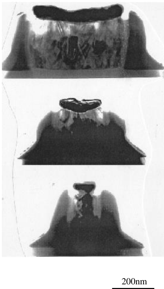
Figure 2-1-9. TEM photograph of cross section through \text{TiSi}_2 -polycide.
