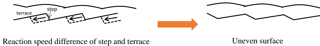
Fig 5.3.3 the simulation of oxidation of SiC epitaxy surface layer
