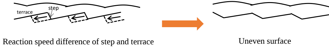
Fig 5.3.3 the simulation of oxidation of SiC epitaxy surface layer
